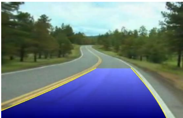
Autonomous vehicles Detect lane markings and road boundaries.
